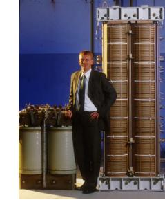
**First 1MVA-HTS** transformer at SIEMENS in 2001. **Function & low** loss was demonstrated.
