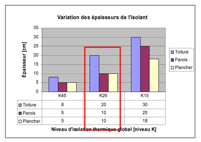
K45 = required insulation level according EPC rules K26 = insulation level of a "low energy" building K15 = insulation level of a "passive" building
